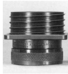
One parallel thread removed to show actual thread angle.
