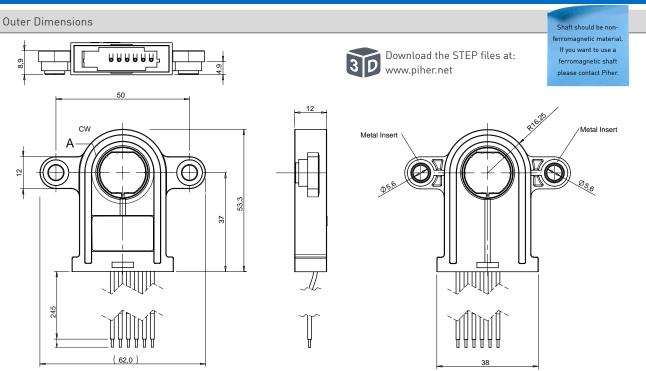
Sensor shown above is the 17mm version with the rotor at zero position. Sensor is delivered at random position. Wires: 0.35mm² TXL SAE J1128
