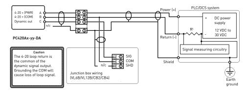
Note: Dynamic output must be galvanically isolated when connected to an on time system.
