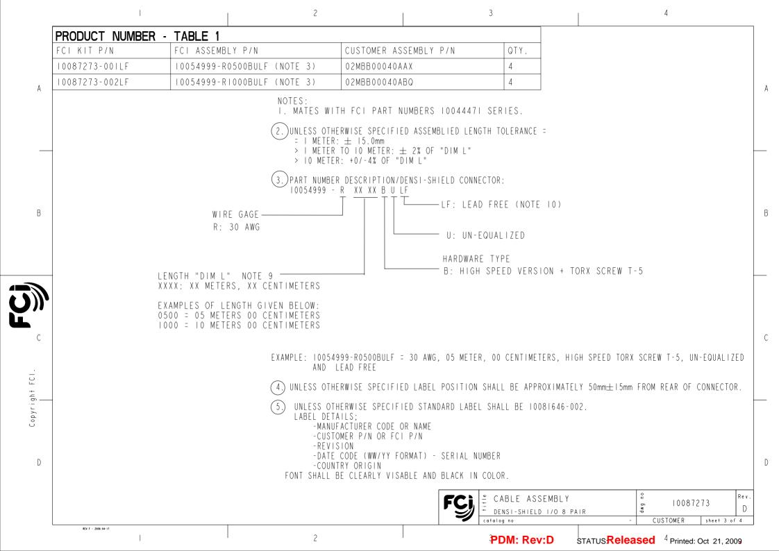
CONNECTOR ASSEMBLIES SHOWN ARE FOR REFERENCE ONLY AND MAY NOT SHOW ALL PART DETAIL. REFERENCE CONNECTOR ASSEMBLY DRAWINGS FOR COMPLETE DETAILS.
