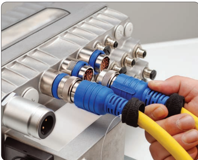
Color-coded thermoplastic bands for visual verification.
