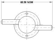
The Quick Calibration Hood is constructed from polypropylene, and provides a convenient means of supplying test gases to the IR600 in the field, for calibration and checking purposes. The assembly push-fits into the central gas access recess of the head, and is designed to accommodate 6 mm ID or ¼" flexible tubing.
