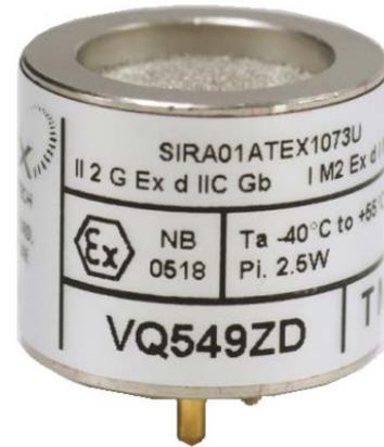
If a flammable gas is present when the bead is heated to about 400 to 500 °C, the gas will oxidise and the resultant release of energy will heat the bead still further. This increase in temperature is detected as an increase in resistance of the coil.
