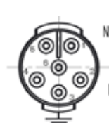
8MF1-PSM L: 85-264 VAC 4, 5, 6: Not connected
