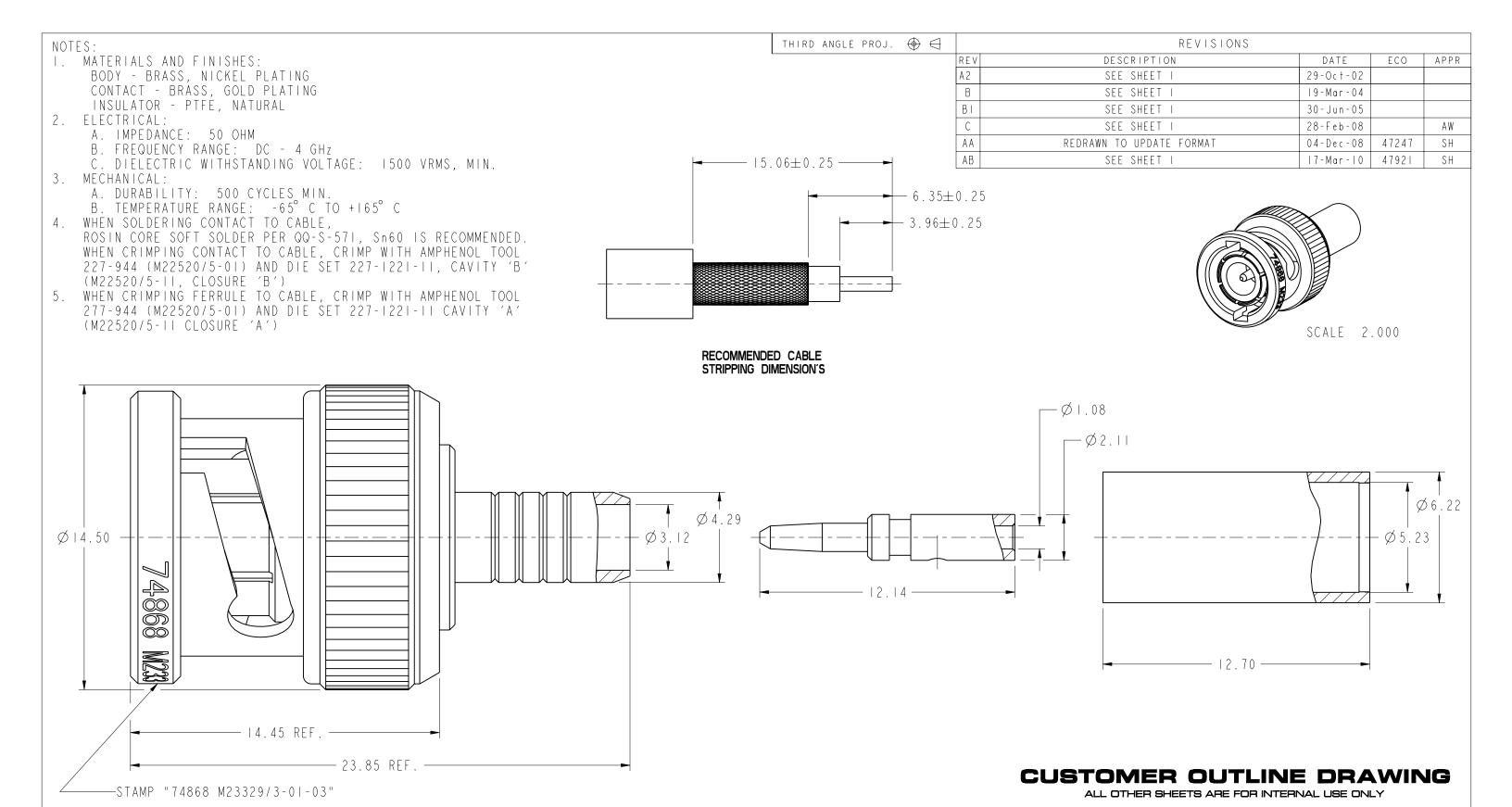
UNLESS OTHERWISE SPECIFIED, DIMENSIONS ARE IN METRIC AND TOLERANCES ARE:  $\pm\,$ 0 . Imm  $\pm\,$ 0.2mm ± 0.3mm NOTICE - These drawings, specifications, or other data (I) are, and remain the
