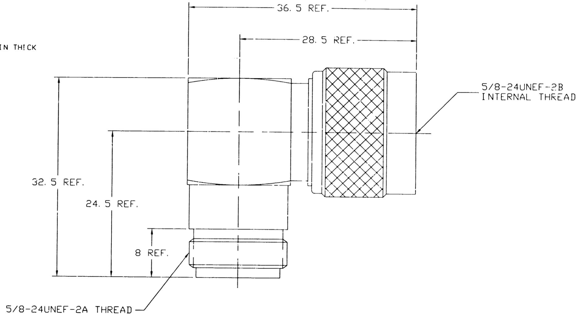
UNLESS OTHERWISE SPECIFIED, DIMENSIONS ARE IN MILLIMETRES AND TOLERANCES ARE:
