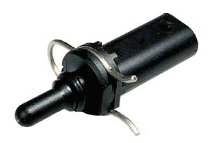
Thermometrics GE-2133 Series of General Fluid Temperature Sensors measures and monitors the temperature of a variety of fluids. The spring clip design secures the sensor in place and provides a quick means for installation and removal.
