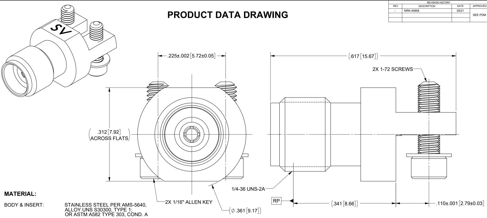
BERYLLIUM COPPER PER ASTM B196, ALLOY No. UNS C17300, TD04 CONTACT:
