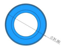
All dimensions are in mm All tolerances are ±0.15mm
