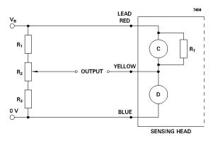
$R_1$  =  $R_3$  = 500 to 5000  $\Omega,\ R_2 \cong R_1/5$
