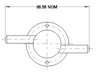
The Quick Calibration Hood is constructed from polypropylene, and provides a convenient means of supplying test gases to the VQ600 in the field, for calibration and checking purposes. The assembly push-fits into the central gas access recess of the head, and is designed to accommodate 6 mm ID or 1/4" flexible tubing.
