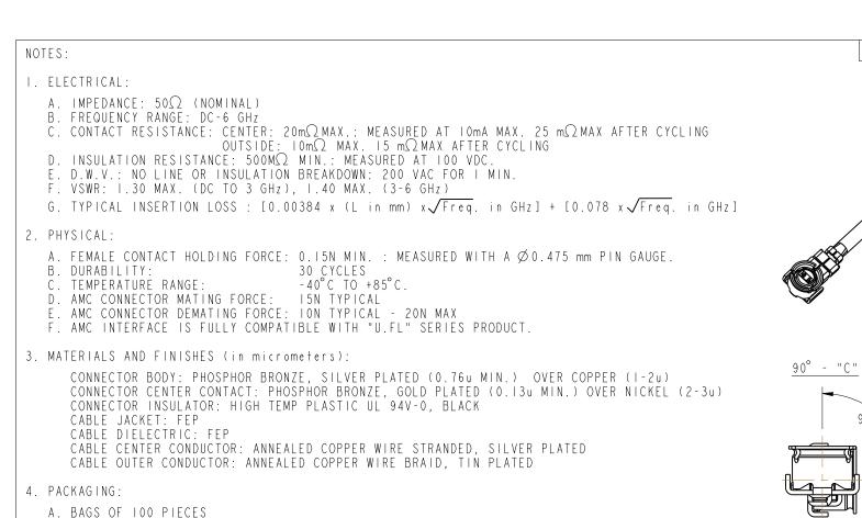
THE ECC OTHERWISE SPECIFIED DIMENSIONS ARE IN METRIC AND TOLERANCES ARE. MATERIAL
