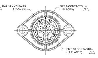
REDUCED DIA. WIRE SEAL SEALED PANEL MOUNT
