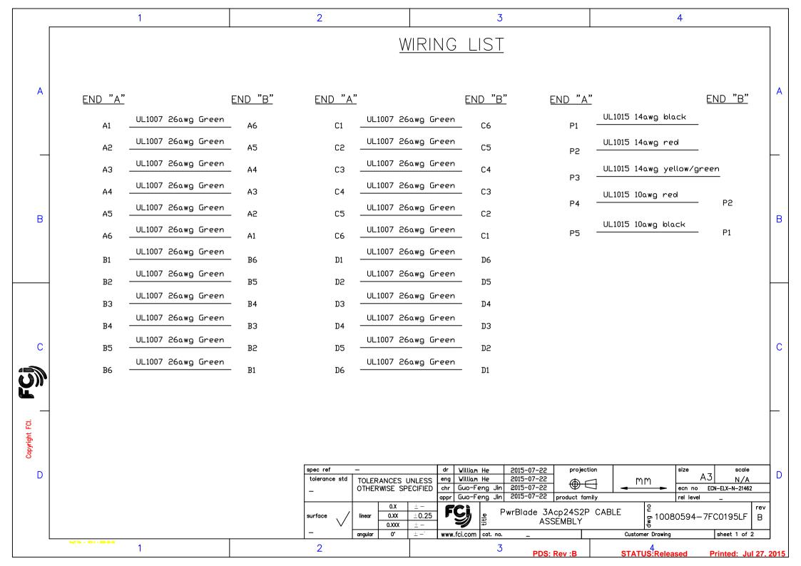
2. UNLESS OTHERWISE SPECIFIED ASSEMBLIED LENGTH TOLERANCE =  $\langle$  = 1 METER: ±15.0mm > 1 METER TO 10 METER: ±2% OF L1 > 10 METER: +0.00% / −4% ΠF L1
