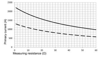
$- U_{C} = \pm 24 \text{ V} - 5 \%$ ,  $T_{A} = 85 \degree C$ ---U<sub>C</sub> = ±15 V -5 %, T<sub>A</sub> = 85 °C
