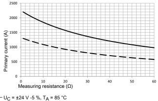
$U_C = \pm 24 \text{ V} - 5 \text{ \%}, \text{ I}_A = 85 \text{ °C}$ ---  $U_C = \pm 15 \text{ V} - 5 \text{ \%}, \text{ T}_A = 85 \text{ °C}$ Primary currents higher than I<sub>PM</sub> only for peak!
