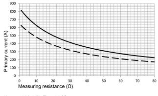
$\begin{array}{c} ---- U_C = \pm 15 \ V \ -5 \ \%, \ T_A = 85 \ ^\circ C \\ ---- V_C = \pm 12 \ V \ -5 \ \%, \ T_A = 85 \ ^\circ C \\ Primary currents higher than \ I_{PM} \ only \ for \ peak! \end{array}$
