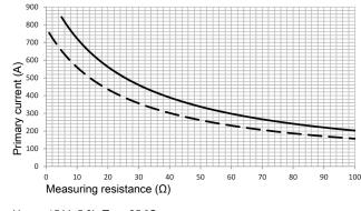
$\label{eq:UC} \begin{array}{l} ---- \mbox{U}_C = \pm 15 \mbox{ V} -5 \mbox{ \%}, \mbox{ T}_A = 85 \mbox{ °C} \\ ---- \mbox{V}_C = \pm 12 \mbox{ V} -5 \mbox{ \%}, \mbox{ T}_A = 85 \mbox{ °C} \\ \mbox{Primary currents higher than } \mbox{I}_{PM} \mbox{ only for peak!} \end{array}$
