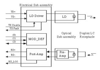
Pin assignment diagram of transceiver
