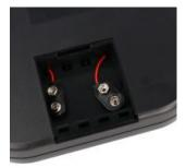
One 9V battery clips rea supplied with S battery door sizes and two clips are
