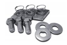
The 1463S is a hardware kit used to mount rack rails and other vertical rack accessories to Hammond cabinets. The  $3/8 \times 16$  spring-loaded nuts install in seconds and simply push-in and rotate to secure in place into the rack cabinet ganging kit "C" channels.
