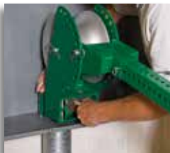
Connect for an upward pull
