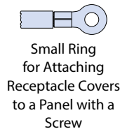
Small Ring for Attaching Receptacle Covers to a Panel with a Screw
