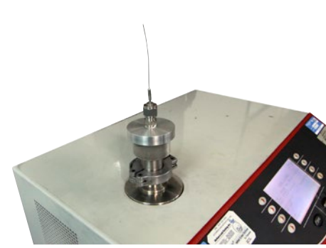
Gas tube helium leak test equipment
