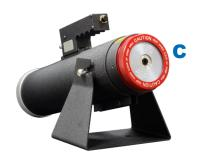
Bench mount pneumatic crimp tool. Heavy duty, four-indent crimp termination. Attach to air supply with quick-disconnect fitting or install 1/4 NPT fitting into tapped port. 90-120 psi air supply. Requires die assemblies and locators, sold separately. Hand actuate with push-button valve trigger on handle. Steel with black wrinkle enamel coating. 13 inches overall length, 9.2 inches tall, 17 pounds (7.7 Kg).
