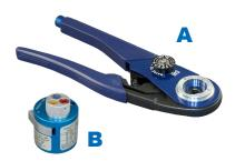
A Crimp tool for use with size #16 and #12 Series 970 pin and socket contacts. Use with turret-type positioner 859-032. 9.75 inches OAL, 1.25 pounds.
