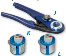
Crimp tool for use with size #20, #16 and #12 power pins. 9.75 inches OAL, 1.25 pounds. Use with M39029/57 and /58 contacts and 809-093 adapters.
