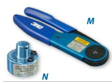
For crimping size #16 shield sleeves. These mil spec approved tools feature a ratchet mechanism to prevent damage from overcrimping. Check calibration with M22520/3 gage.
