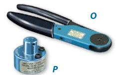
For crimping size #12 shield sleeves. These mil spec approved tools feature a ratchet mechanism to prevent damage from overcrimping. Check calibration with M22520/3 gage.
