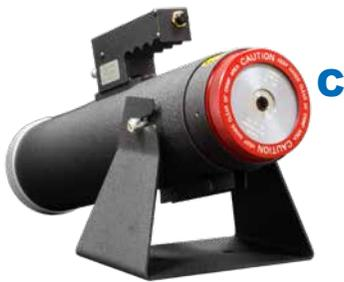
**C** Bench mount pneumatic crimp tool. Heavy duty, four-indent crimp termination. Attach to air supply with quick-disconnect fitting or install 1/4 NPT fitting into tapped port. 90-120 psi air supply. Requires die assemblies and locators, sold separately. Hand actuate with push-button valve trigger on handle. Steel with black wrinkle enamel coating. 13 inches overall length, 9.2 inches tall, 17 pounds (7.7 Kg).
