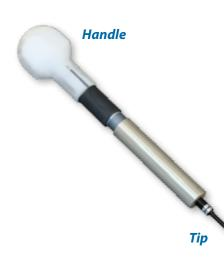
Check for properly seated contacts with this spring-loaded tester. Apply the tool tip to the mating end of a contact. Push on the handle until the spring compresses to the recommended force. A visual indicator shows full compression. The contact is properly retained if it is not displaced. Adjust handle to appropriate settings:
