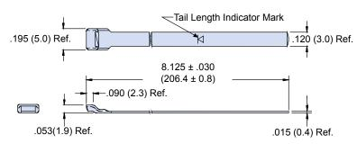
The 600-057 Micro Band is precision constructed of 300 Series SST/Passivate, and designed for use with the 600-061 Hand Banding Tool or the 600-068 Pneumatic Banding Tool. Double-wrapped bands will accommodate diameters up to approximately .88 inches (22.4). Bands may be ordered flat (600-057), or precoiled (600-057-1). Bands come bagged and tagged in quantities from 1 to 100.
