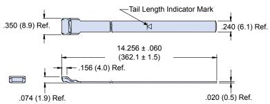
The 600-052 Standard Band is precision constructed of 300 Series SST/Passivate and designed .240 (6.1) Ref. for use with the 600-058 Hand Banding Tool or the 600-067 Pneumatic Banding Tool. Double-wrapped bands will accommodate diameters up to approximately 1.8 inches (45.7). Bands may be ordered flat (600-052) or precoiled (600-052-1). Bands come bagged and tagged in quantities from 1 to 100.
