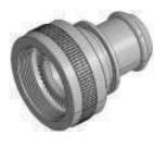
This is another method of termination of screens. A high quality band will do the job in this back shell. Tempered bands are tightened over the shields, which is pulled over the banding area, using special assembly tools. Suitable over cover by heat shrink boot or some other method as chosen by the designer could be used. Both crimp ring and banded terminations give a low DC resistance.
