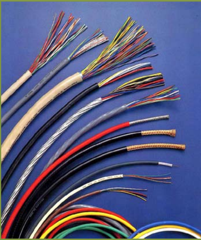
The heart of every interconnect cable assembly is the multi-conductor cable. As early in the application development process as possible it is critical to document the wire gauges, core type, insulation/dielectric materials, media types (copper, aluminum or optical), shielding (individual conductor and overall), jacketing, and all other elements that contribute to the mechanical and dimensional properties of the cable. By the way, Glenair's cable shop can supply the cable, particularly for unusual or short run applications.
