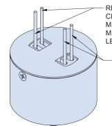
REDUNDANT INITIATION CIRCUIT WIRES IAW MS22759/44-20-0 AND MS22759/44-20-2. LENGTH = 18 INCHES MIN.
