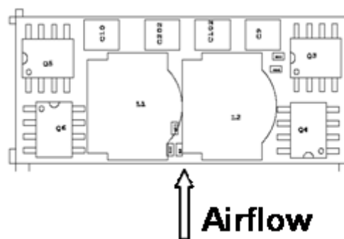
Figure 34. Airflow direction for thermal testing.
