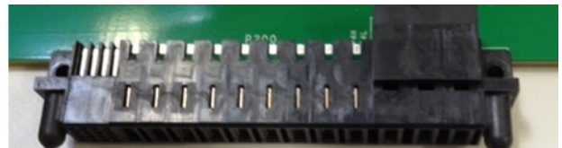
Figure 23 - Mating connector with input exiting flying leads
