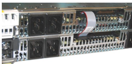
Figure 15 - Shelf-to-shelf ribbon cable of connector J2
