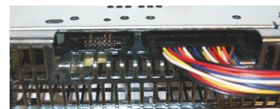
Figure 14 - Control cable plugged into the J1 connector
