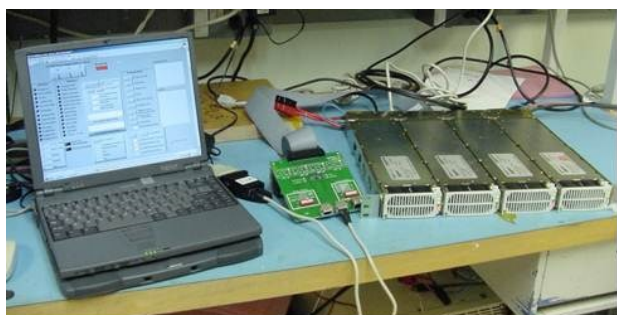
Figure 10 -Test setup using a OmniOn J85480 shelf
