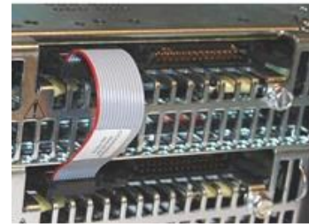
Shelf-to-shelf cable connection (part # CC848848952)
