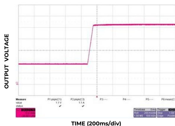
Figure 4. Main output: Output changed from 18V to 52V; commanded via I 2 C. (For reference)
