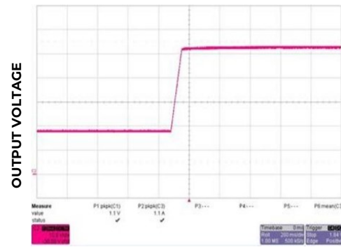
Figure 4. Main output: Output changed from 18V to 52V; commanded via I 2 C
