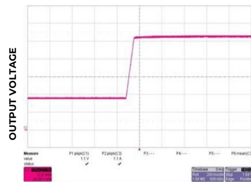
Figure 4. Main output: Output changed from 18V to 52V; commanded via I 2 C
