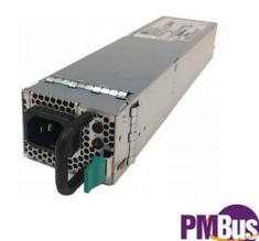
The MPR0712 series is a 700W ACDC power supply with a power density of 23W/in3 at an efficiency of 94% @ 50% Load. The smaller depth of 9" would be conducive for mid plane system architectures and in applications that are limited in space. MPR0712 uses the industry standard PMBus® compliant I2C communications bus and offers a full range of control and monitoring capabilities. The SMBAlert signal pin automatically alerts customers of any state
