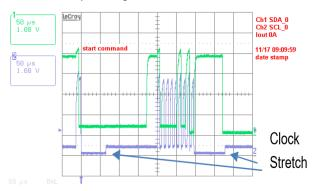
**I<sup>2</sup>C Bus Lock-Up detection:** The device will abort any transaction and drop off the bus if it detects the bus being held low for more than 35ms.
