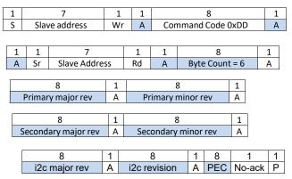
**Read\_run\_timer [0xD6]:** This command reads back the recorded operational ON state of the rectifier in hours. The operational ON state is accumulated from the time the rectifier is initially programmed at the factory. The rectifier is in the operational ON state both when in standby and when it delivers main output power. Recorded capacity is approximately 10 years of operational state.
