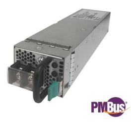
The MPR0712DC series provides high efficiency isolated power from the DC input mains. The industry standard PMBus<sup>®</sup> compliant I2C communications bus offers a full range of control and monitoring capabilities. The SMBAlert signal pin automatically alerts customers of any state change within the power supply.
