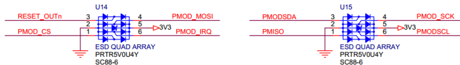
Figure 38 - Pmod Connector ESD Protection Schematic
