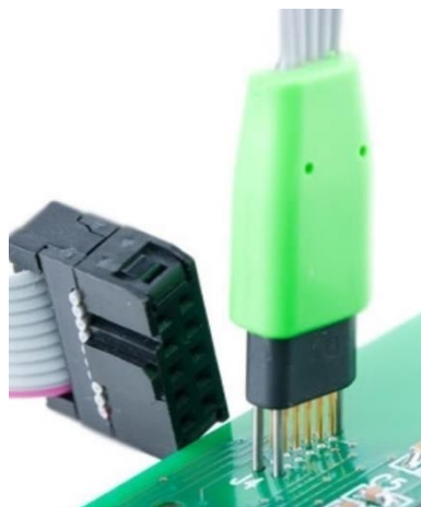
Figure 41 - Tag Connect Header inserted into PCB
