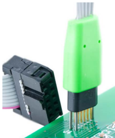
Figure 55 - Tag Connect Header inserted into PCB
