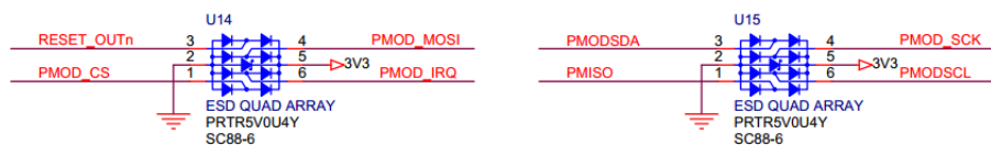
Figure 48 - Pmod Connector ESD Protection Schematic
