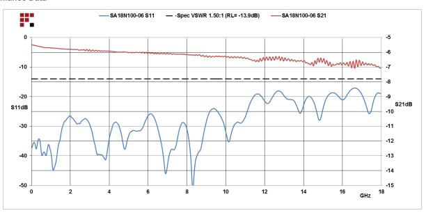
6 dB Fixed Attenuator N Male (Plug) to N Female (Jack) Up to 18 GHz Rated to 100 Watts, Heatsink Body, 1.45 VSWR from Fairview Microwave is in-stock and available to ship same-day. All of our RF/microwave products are available off-the-shelf from our ISO 9001:2008 certified facilities in Lewisville, Texas. Fairview Microwave is RF on-demand.
