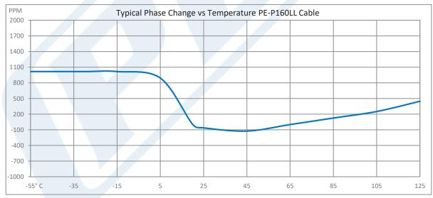
Click the following link (or enter part number in "SEARCH" on website) to obtain additional part information including price, inventory and certifications: Temperature Conditioned SMA Male to N Male Low Loss Cable 200 cm Length Using PE-P160LL Coax PE3M0186-200CM
