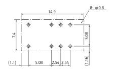
NAL-D (double winding latching type)
