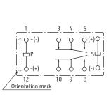
PC board mounting hole layout (BOTTOM VIEW)
