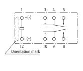
PC board mounting hole layout (BOTTOM VIEW)
