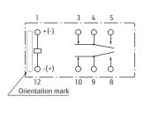
PC board mounting hole layout (BOTTOM VIEW)
