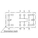
PC board mounting hole layout (BOTTOM VIEW)
