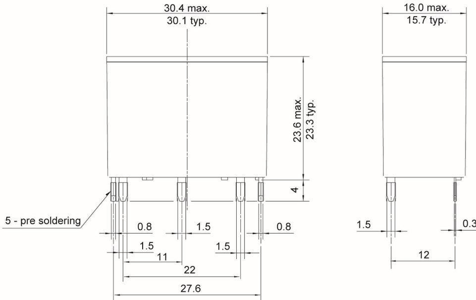
Dimensions of the terminals do not include thickness of pre-solder.
